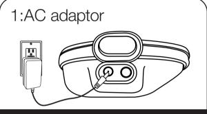
Connect AC adaptor to the DC jack on the left of the unit and plug the other end into a working wall socket. The internal battery (and docked iPod/iPhone) will charge.
